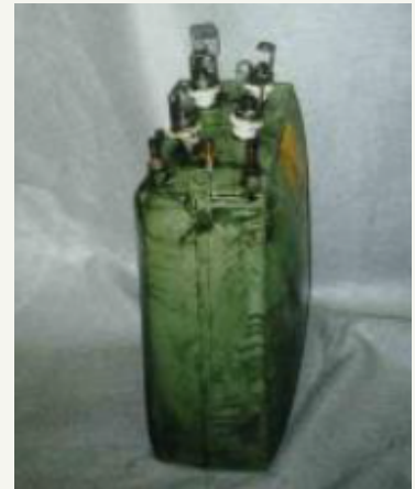
Figure 5: Convex or swollen shape capacitor
