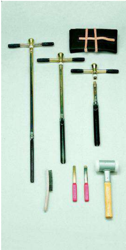
Manual work to gouge debris-rich soils
