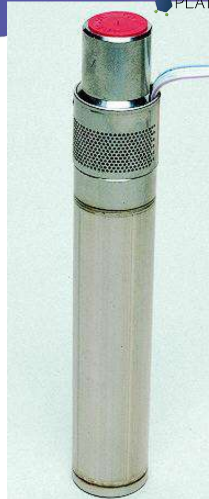
Impellor pump Sampling dept max 80 m
