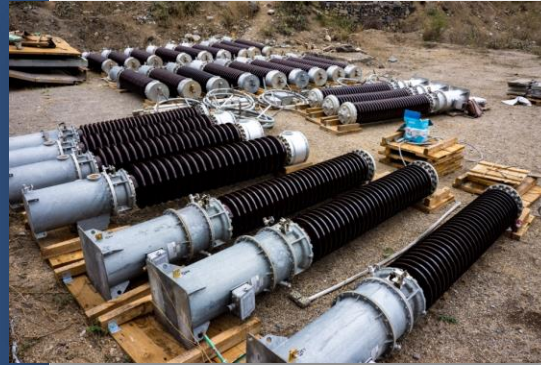
Capacitors voltage transformers (Aroclors A-1242, A-1254 A-1260)
