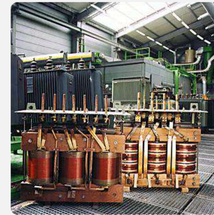
Separation of cores and casings. Source: Capo A., BRS/UNITAR Regional PCB Webinar (2025). https://pcb.unitar.org/webinar-series/regional/webinar-3/
